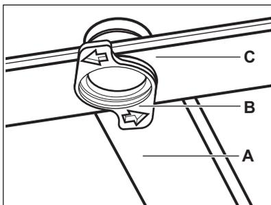
1. Release the stoppers on the sides of the sliding rails of the cutlery drawer and pull the drawer out.
