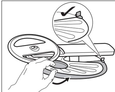
7. Reassemble the filters (B) and (C).
