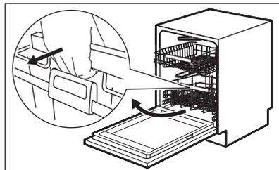
The basket is automatically locked on the upper level.
