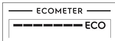
The ECOMETER indicates how the programme selection impacts energy and water consumption. The more bars are on, the lower the consumption is.
