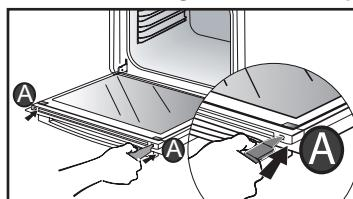
Remove the glass panel. The door consists of two additional glass panels, with a black rubber spacer at each corner.
