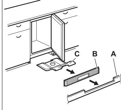
1. Remove the plinth (A), then the ventilation grid (B).
