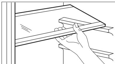
The walls of the refrigerator are equipped with a series of runners so that the shelves can be positioned as desired. For better use of space, the front half-shelves can lie over the rear ones.
