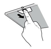
2. Take the metal grease filter out of the holder.
