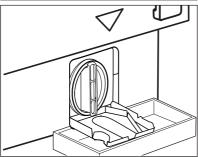
2. Place a suitable bowl below the drain pump access to collect the water that flows out. Always keep a rag nearby to dry up any water spillages when removing the filter.
