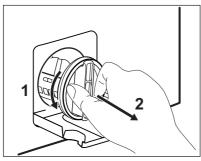
6. Turn the filter anti-clockwise to remove it
