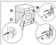
Make sure that the plate with magnet is on the upper position.
