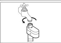
**5.** Connect the water inlet hose to the cold water tap with 3/4 thread.
