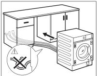
Before proceeding with appliance building in, bring it near the recess and preposition the inlet hose, the drain hose and the mains cable.
