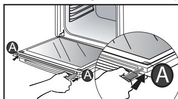
Remove the glass panel. The door consists of two additional glass panels, with a black rubber spacer at each corner.
